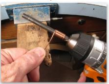
If you need a few jump rings the same size, it's easy to grab a round rod and wind as many as you need. But when you need a lot of them, some form of winder saves a lot of time. A variable speed screw gun makes quick work of winding the coils. Screw guns are quite inexpensive at discount stores and are remarkably handy for odd jobs in the shop and around the house.
