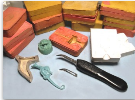
SHARP KNIVES FOR CUTTING MOLDS
