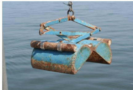
Figure 1. Peterson grab used to pull muddy sediments from the ocean floor with 2015 Dauphin Island Marine Geology class. Lead weights drop the grab to the bottom where it triggers and “bites” the seafloor (Photo Michael Gibson, 2015).
