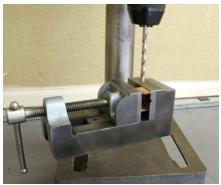
You can find them at stores that carry machine tool supplies. My feeling is that the best ones are made from steel. And I like the ones with V grooves cut into the jaw plates to help hold a punch straight up or to hold a rod horizontal. To find a supplier, search on "vise" or "drill press vise" at micromark.com, use-enco.com, smallparts.com, grizzly.com, sears.com.
