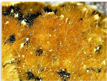
Figure 2. Cacoenite needles coating beraunite, magnification is 15X. This specimen is from Three Oak Gap, at an abandoned manganese claim, in Polk County. Self collected.
