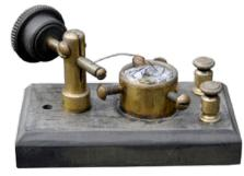
The "cat's whisker" crystal detector (see picture) in crystal radios was actually an improved version, developed by other people, but it was based on Braun's work. It consists of a thin wire that lightly touches a crystal of semiconducting mineral (usually
