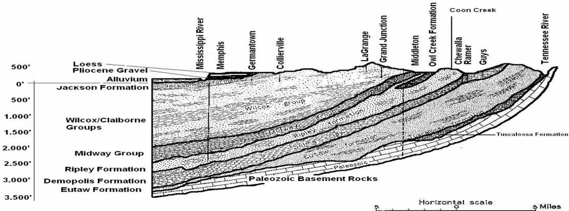
Figure 6. Cross section of The Mississippi Embayment Although some of the stratigraphy is dated, this section shows how sediments filled a shallow around 75 million years ago. The trough formed by rifting when North America almost pulled apart hundreds of millions years earlier. The vertical scale of the deposits are greatly exaggerated. Modified from Francis G. Wells 1933 "Ground Water resources of Western Tennessee", United States Geological Survey [Water-Supply Paper 656](#), plate 5.
